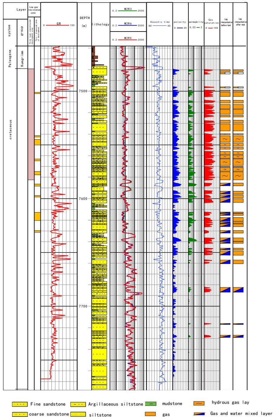
Fig. 3 Typical curve of low-resistivity stratum in Keshen area
