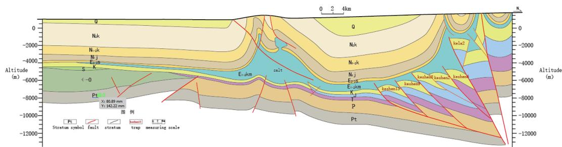
Fig. 2 Geologic analytic model of Kelasu structural belt
