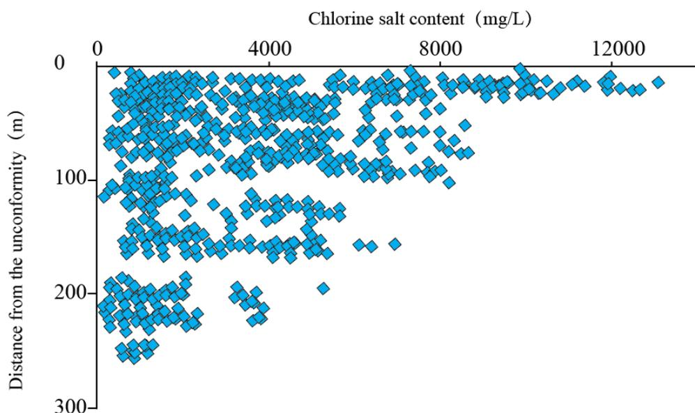
Fig. 4 Relationship between chlorine content and distance from the unconformity surface
